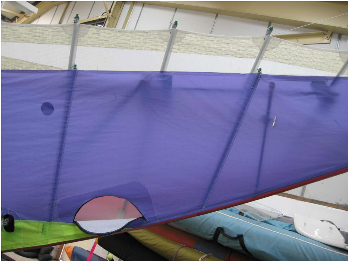
Rigging stage 12 – correct positioning of washout rods.
